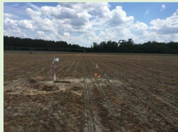
Figure 2. Corn strip planted into cover crop over drain gauge and lysimeter (orange flags in foreground) installation site.
