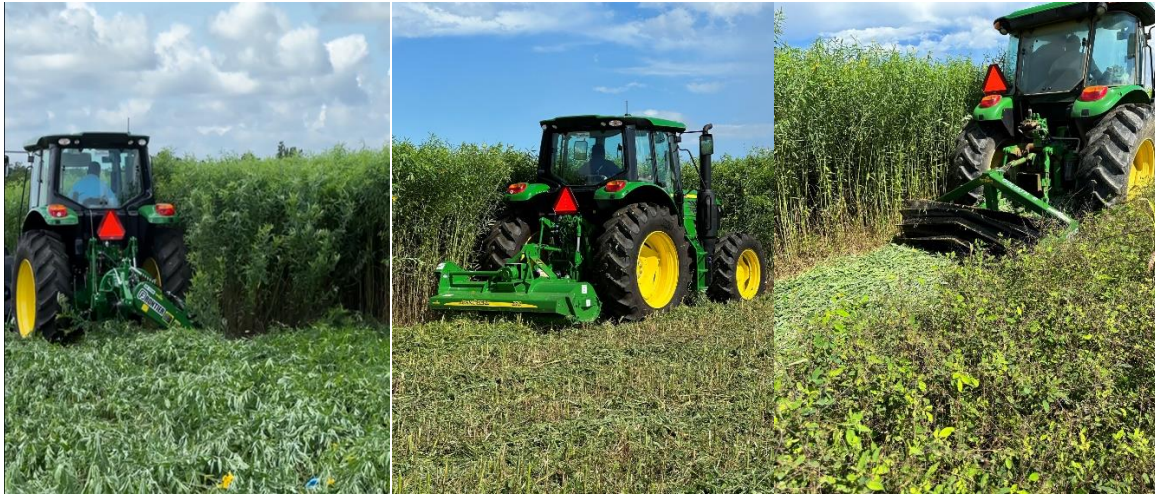
Fig. 2. TREC cover crop termination with sickle bar mower, flail mower, and rolling crimper.
